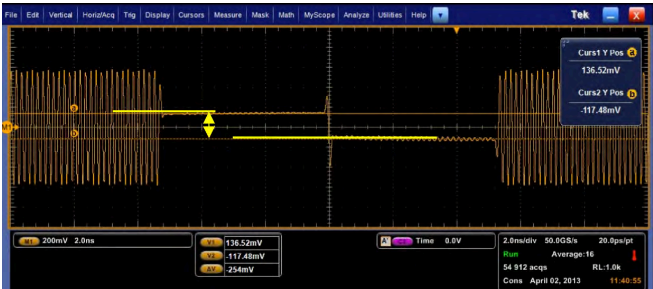
FIGURE 41. MEASURED NON-TRANSITION AMPLITUDE (EXAMPLE 254mV)
