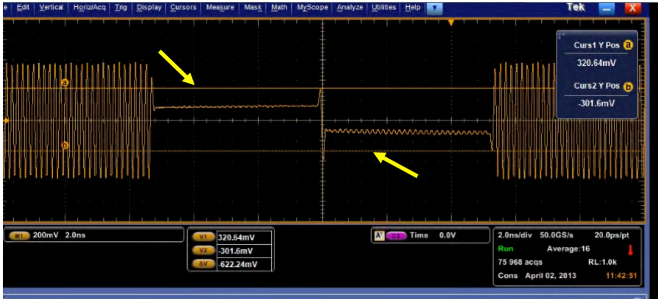
FIGURE 42. MEASURED PRESHOOT AMPLITUDE (EXAMPLE 622mV)
